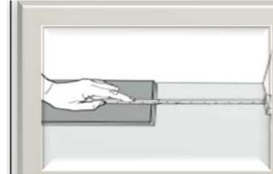
The last piece in the row should be cut to length while maintaining the 10mm expansion gap along the perimeter of the room.
