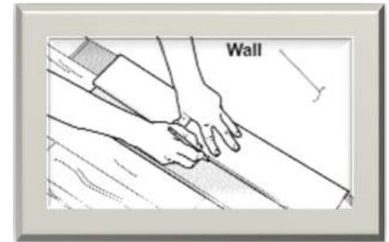
The last row (possibly the first row) plank width should be no less than 50mm (2") on the long seam. Remember to allow for a gap of 10mm (3/8") to the wall.
