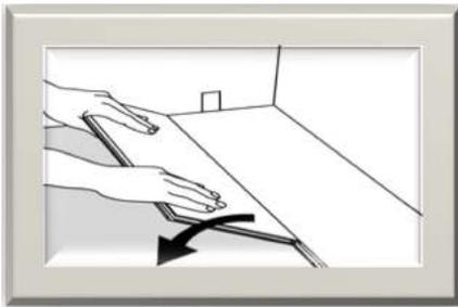
Cut a piece that is at least 5.9" or 150mm shorter than the first plank to start the second row or use the cut off from the previous row, keeping in mind the length requirements above.
