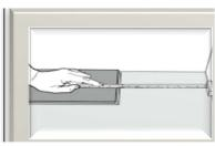
The last piece in the row should be cut to length while maintaining the 10mm expansion gap along the perimeter of the room.
