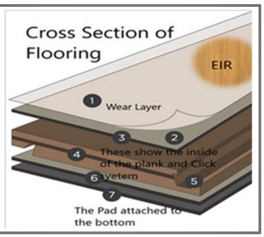
**Pad Attached** – Indicates that there is a pad attached to the core. This pad will increase sound deadening and make the product softer under foot. Pad thickness will vary along with type of pad will vary.
