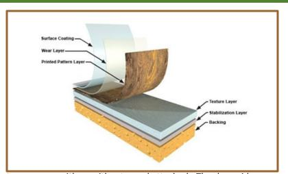
Because it is more rigid than LVT, often times these products can come with or without a pad attached. The downside of WPC is that it is not as dense as LVT or SPC. Since it has pockets throughout the core, it tends to shrink and swell with temperature changes. These products can be produced in both ABA and Direct Print.
