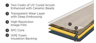
By using a stone and vinyl combination in the core the end result is the most rigid product in the category. SPC's are also the densest products in the category often times exceeding 3000 psi. Because stone does not shrink and swell with temperature SPC is the most dimensionally stable product in the category as well. It can be used in cabins, 3 season rooms, and areas where you could only put tile or carpet in before. These products can be produced in both ABA and Direct Print.
