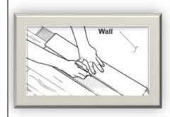
The last row (possibly the first row) plank length should be no less than 30mm (12") on the long seam. Remember to allow for a gap of 10mm (3/8") to the wall.
