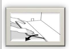
Cut a piece that is a least 5.9" or 150mm shorter than the first plank to start the second row or use the cut off from the previous row, keeping in mind the length requirements above.
