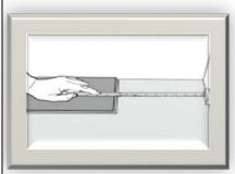
The last piece in the row should be cut to length while maintaining the 10mm expansion gap along the perimeter of the room.
