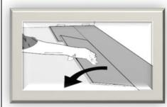
To install the remaining planks in the second row, first align the long edge tongue into the groove of the previous row at a shallow angle. Slide the piece to the left until the piece meets the previously installed piece.
