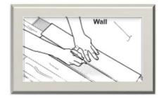
The last row (possibly the first row) plank width should be no less than 50mm (2") on the long seam.
