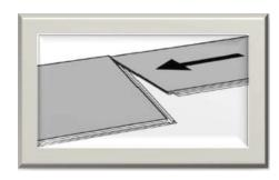
Install the second piece in the first row by laying the short end tongue onto the previously installed piece short-end groove.
