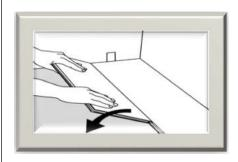
Cut a piece that is a least 5.9" or 150mm shorter than the first plank to start the second row or use the cut off from the previous row, keeping in mind the length requirements above.
